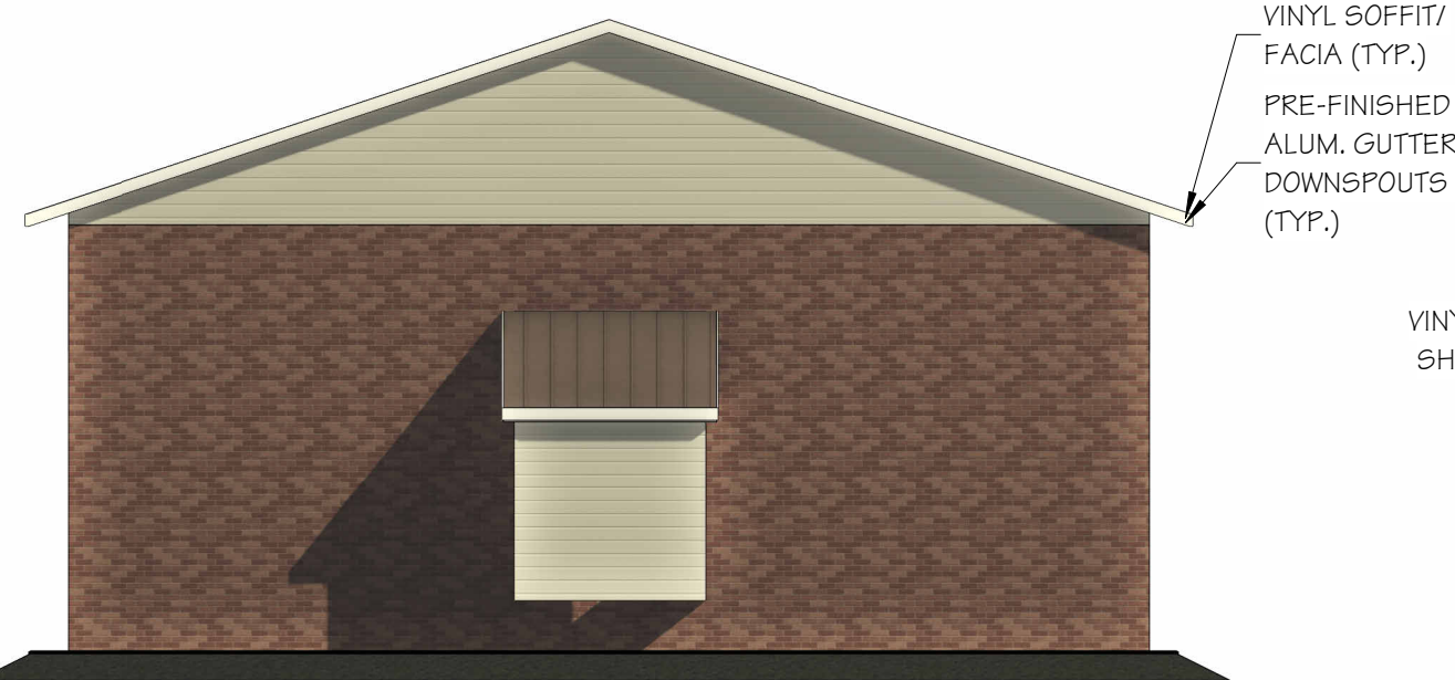
10 BLDG. TYPE "H" TYP. SIDE ELEVATION API3 SCALE: 1/8" = 1'-0"
