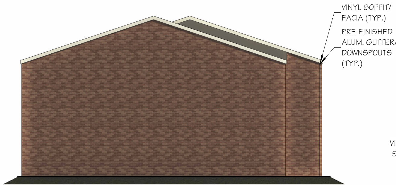
4 BLDG. TYPE "FX" TYP. SIDE ELEVATION API3 SCALE: 1/8" = 1'-0"
