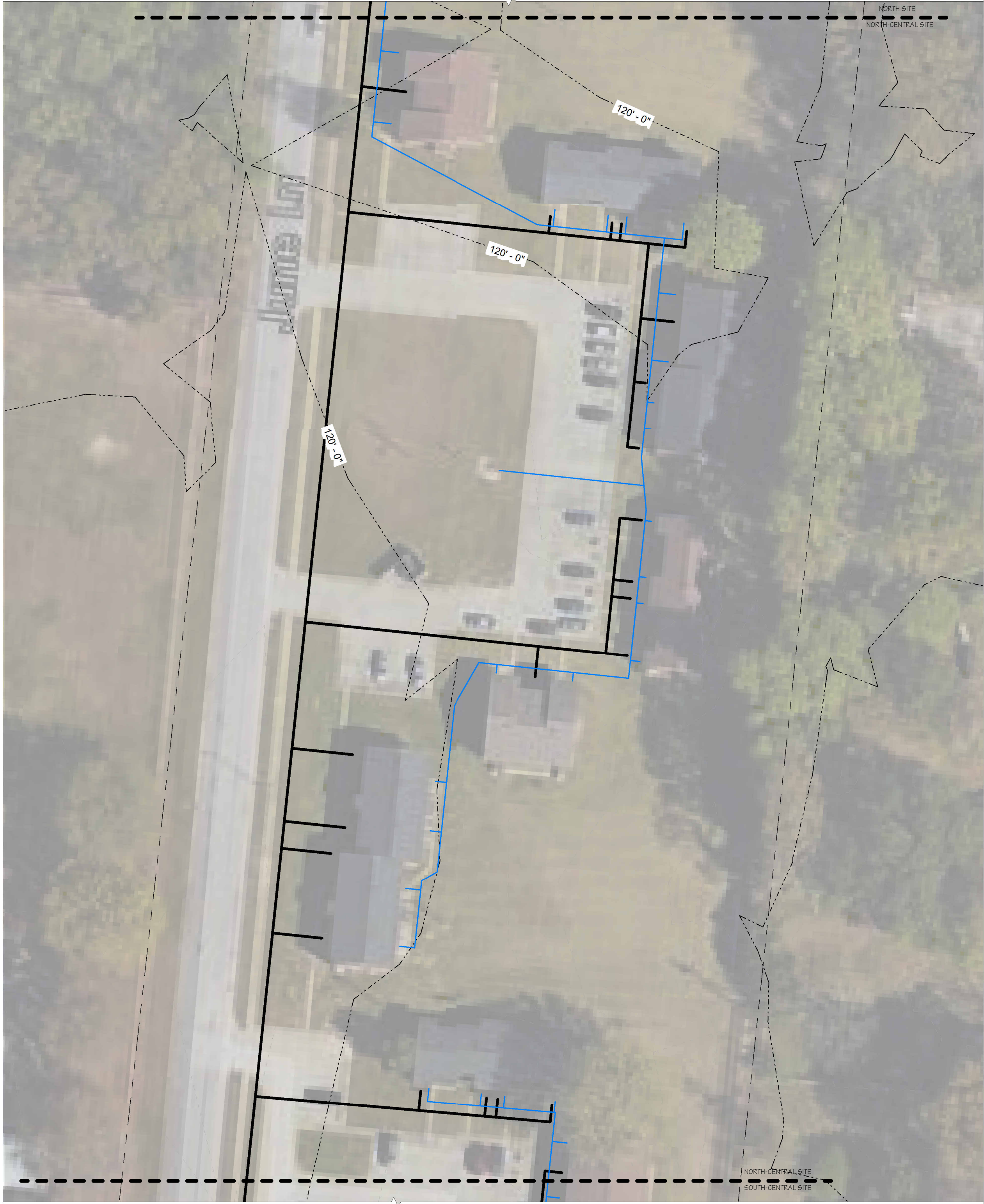
2 AP3 EXISTING UTILITY PLAN - NORTH-CENTRAL SCALE: 1" = 40'-0"
