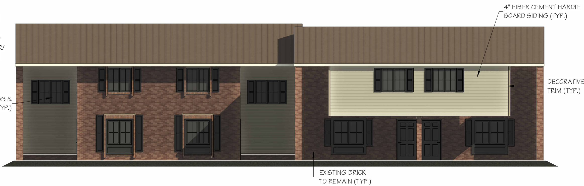
8 BLDG. TYPE "G" FRONT ELEVATION API3 SCALE: 1/8" = 1'-0"
