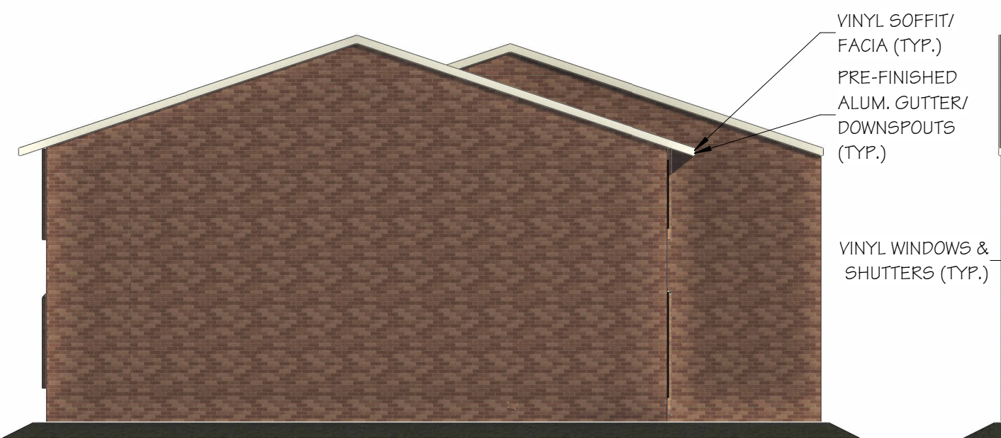
7 BLDG. TYPE "G" TYP. SIDE ELEV. API3 SCALE: 1/8" = 1'-0"
