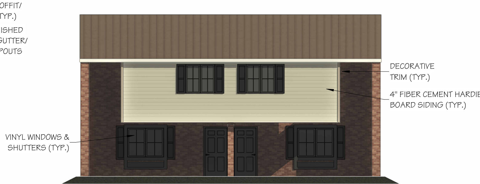
2 BLDG. TYPE "F" FRONT ELEVATION API3 SCALE: 1/8" = 1'-0"
