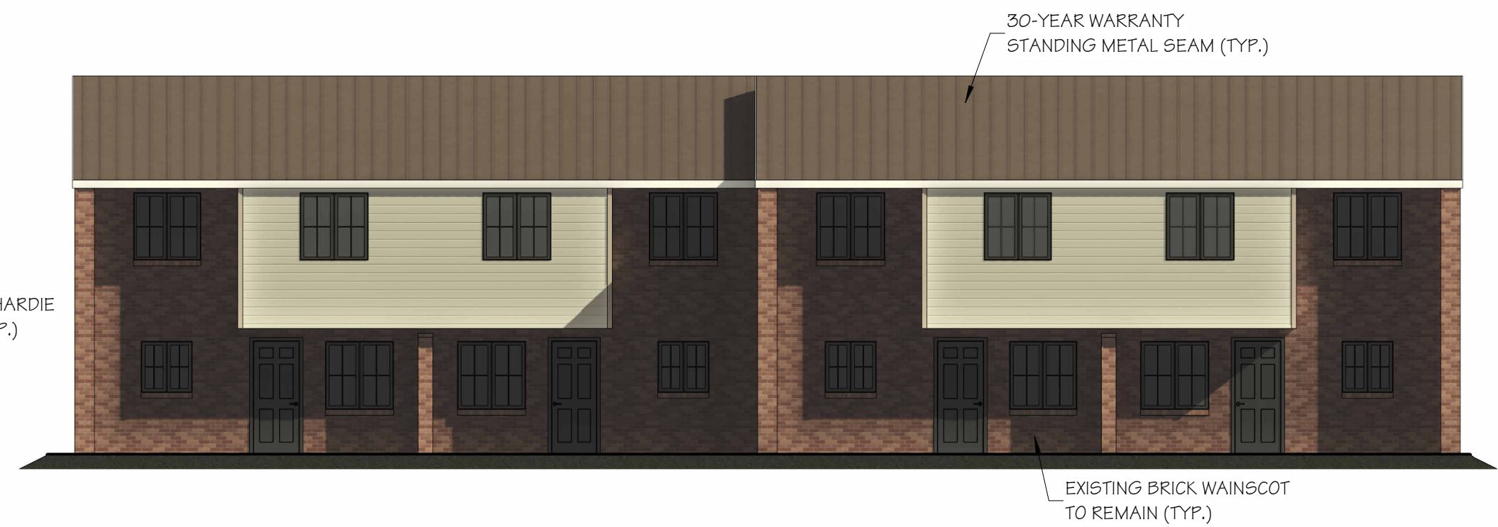
6 BLDG. TYPE "FX" REAR ELEVATION API3 SCALE: 1/8" = 1'-0"
