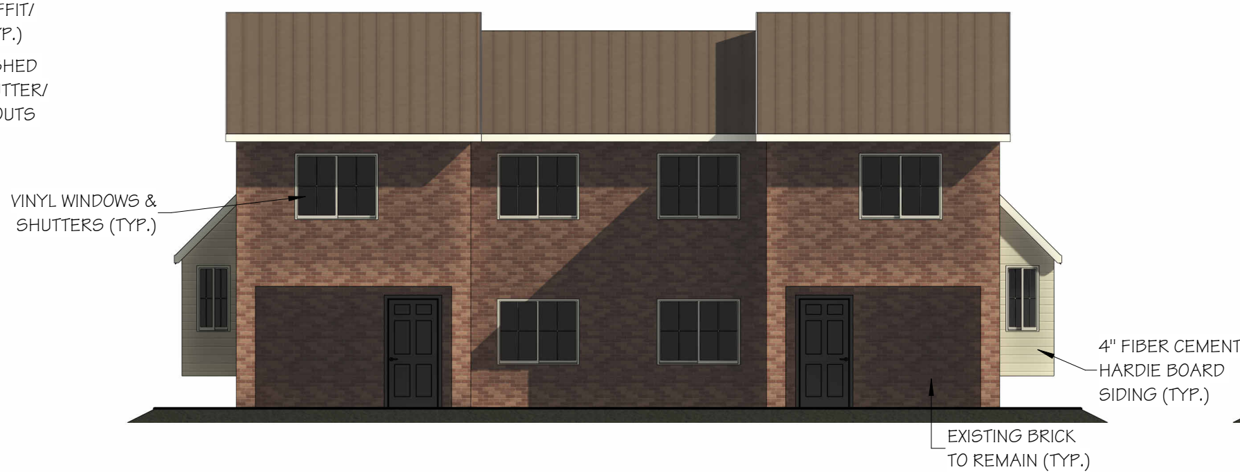
11 BLDG. TYPE "H" FRONT ELEVATION API3 SCALE: 1/8" = 1'-0"
