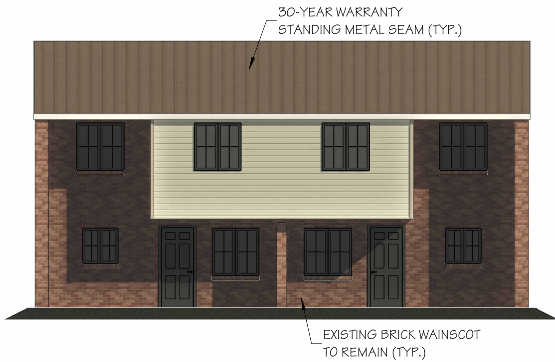
3 BLDG. TYPE "F" REAR ELEVATION API3 SCALE: 1/8" = 1'-0"
