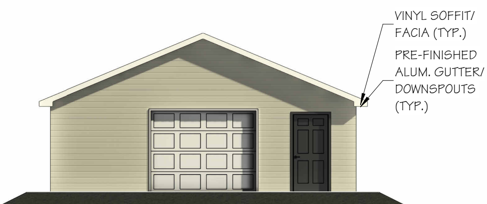
5 AP21 SCALE: 1/8" = 1'-0" MAINT. BUILDING FRONT ELEVATION
